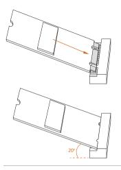
Align and gently insert the M.2 SSD module into the M.2 slot. Please be aware that the M.2 SSD module only fits in one orientation.
