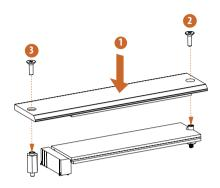
Tighten the screws with a screwdriver to secure the module (if your M.2 SSD module is Type 2280) and M.2 heatsink into place in the order shown. Tighten screw opposite the M.2 connector first (2), and then tighten the one next to the M.2 connector (3).
