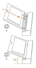
Gently insert the WiFi/BT PCIe WiFi module or Intel\* CNVi (Integrated WiFi/BT) into the M.2 slot. Please be aware that the module only fits in one orientation.
