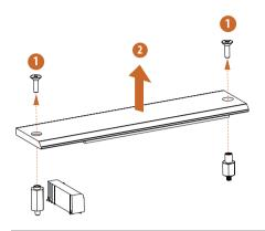
Before installing a M.2 SSD module, please loosen the screws to remove the M.2 heatsink.
